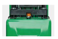
There are safety guardrails on the left and right sides. The guardrails are equipped with detection switches. The vehicle cannot work until the guardrails are put down.
