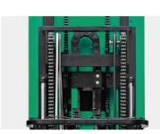
The mast chain with a safety factor of 10 times is equipped with a chain safety
